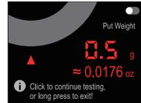
Imbalanced: Weigh the balancing putty to match as indicated on display and shape the putty into a ball if needed. Affix the weight on the tire as the notch arrow indicates at the bottom plate.
