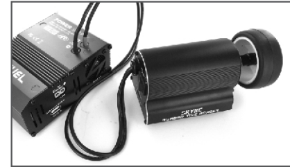
3. Connect tire sander to power supply or 2S LiPo battery
