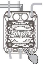
4. Pull the throttle trigger to full throttle and hold it until you hear one beep, indicating that the full throttle calibration is complete.
